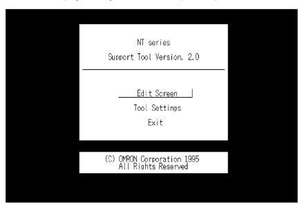
➡ Select "Tool Settings" in the Main Menu to display the "Tool Settings" screen. Settings of PT type, memory size, direct connection are made in this screen. Refer to "Setting the support tool for use with the NT600S" on the previous page.
